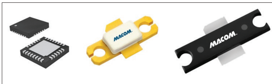
Figure 6: Co-planar (left) packages tend to feature plastic overmoulded parts that trim cost, but impair heat extraction when they are used in PCB circuits. Multi-level packages made from metals and ceramics address this, because the bottom of the package can be in contact with the carrier. However, this approach is expensive. Multi-level plastic overmould parts made by MACOM offer the best of both worlds, combining low cost with good thermal management.
