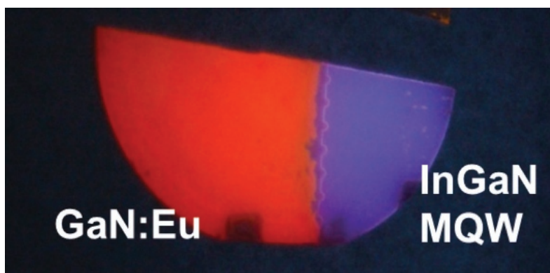
Figure 4. Monolithic integration of blue and red emitting regions on the same LED wafer.
